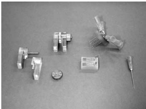
Figure 2 An example of plate and needle electrodes, as constructed at our institution. The plate electrodes are constructed of copper plates mounted on non-conductive material. The screw fixes the two plates in parallel position and different gaps can be obtained by combining plates mounted at different widths. The needle electrodes consist of parallel arrays of hypodermic needles inserted into a custom-made platform that ensures good electrical contact as well as stability and parallelism. We have used this type of electrodes both for in vivo work and in the treatment of patients. When performing in vivo electroporation, particular attention should be paid to E-field distributions. E-field calculations for the electrodes shown are presented in Gehl et al. (1999).
